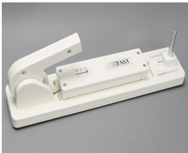
Fig 4. Fundamentals of Arthroscopic Surgery Training (FAST) knot tester. The suture loop is positioned on the 2 tines, and the handle allows for controlled application of 15 lb of longitudinal load.
