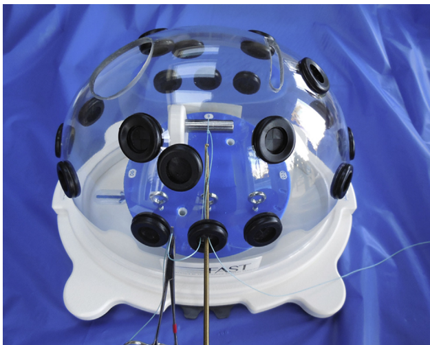
Fig 1. Fundamentals of Arthroscopic Surgery Training (FAST) base station with knot-tying mandrel and lucent dome for skills rehearsal under direct visualization.
