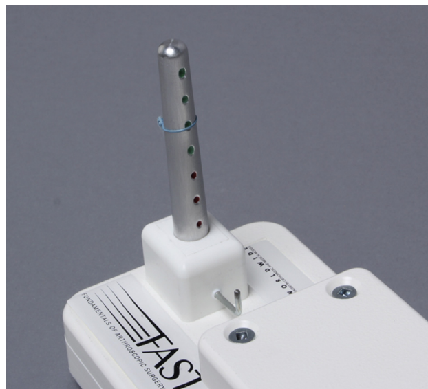
Fig 3. Conical loop sizer of Fundamentals of Arthroscopic Surgery Training (FAST) knot tester. The first mark indicates zero loop expansion, and each subsequent mark reflects 1 mm of additional loop expansion compared with the knot-tying mandrel.
